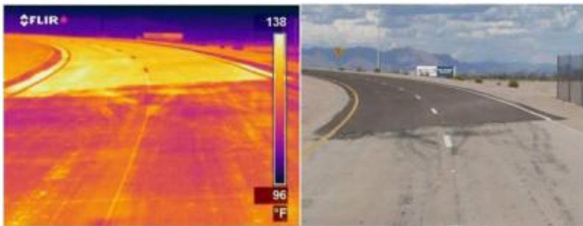
Figure 17: Thermal Infrared Vision of cool pavements compared to a normal asphalt road
