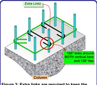
Figure 3: Extra links are required to keep the concrete in place – 180° links are necessary to prevent the 135° tie from bulging outwards.
