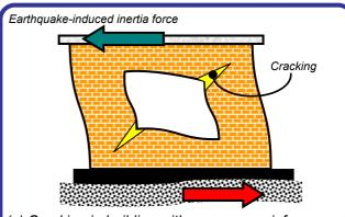
(a) Cracking in building with **no** corner reinforcement
