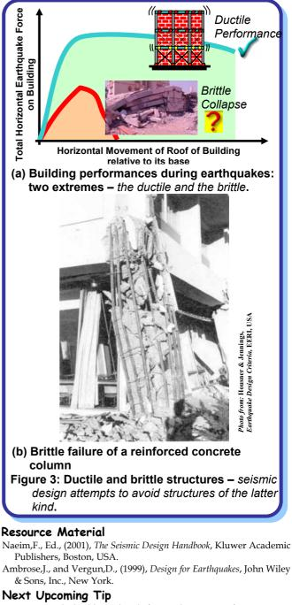
How to make buildings ductile for good seismic performance?
