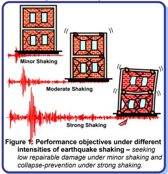
Thus, after minor shaking, the building will be fully operational within a short time and the repair costs will be small. And, after moderate shaking, the building will be operational once the repair and strengthening of the damaged main members is completed. But, after a strong earthquake, the building may become dysfunctional for further use, but will stand so that people can be evacuated and property recovered.
