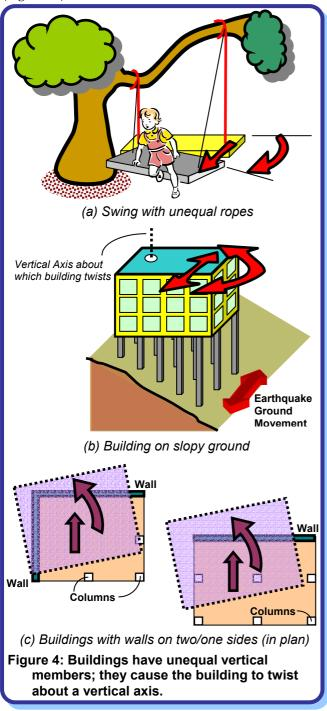
Buildings that are irregular shapes in plan tend to twist under earthquake shaking. For example, in a propped overhanging building (Figure 5), the overhanging portion swings on the relatively slender columns under it. The floors twist and displace horizontally.
