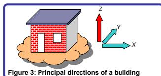
However, horizontal shaking along X and Y directions (both + and – directions of each) remains a concern. Structures designed for gravity loads, in general, may not be able to safely sustain the effects of horizontal earthquake shaking. Hence, it is necessary to ensure adequacy of the structures against horizontal earthquake effects.
